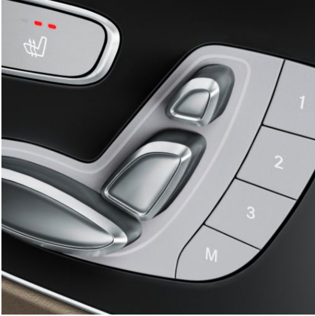
Front seats electrically adjustable with memory function
